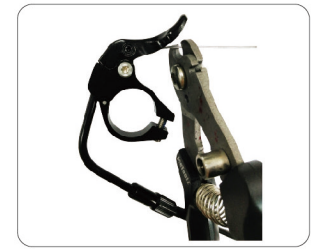
8. Push the lever for 5-10 times to eliminate possible cable loose. 9. Loosen the screw and pull the cable once again until it is tight, fix the screw with 2mm allen key.
