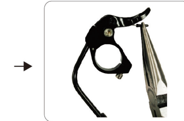
10. Slide the cable into the guide under the lever, cut the cable in appropriate length and fix the cable end.
