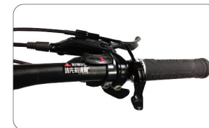
11. Use 3mm hex allen key to fix the clamp lever on the handlebar.
