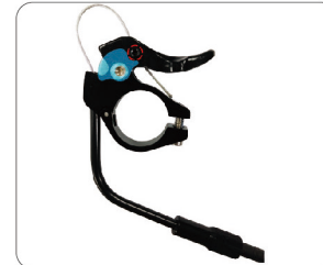
6. Put the nut into the lever with screw set at the left side of lever. ⚠ The nut should be positioned on the curve part of the center blade.
