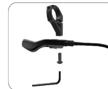
6. Put the nut into the lever with screw set at the left side of lever. ⚠ The nut should be positioned on the curve part of the center blade.
