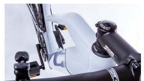
The special profile of the top tube supports an additional rigidity.
